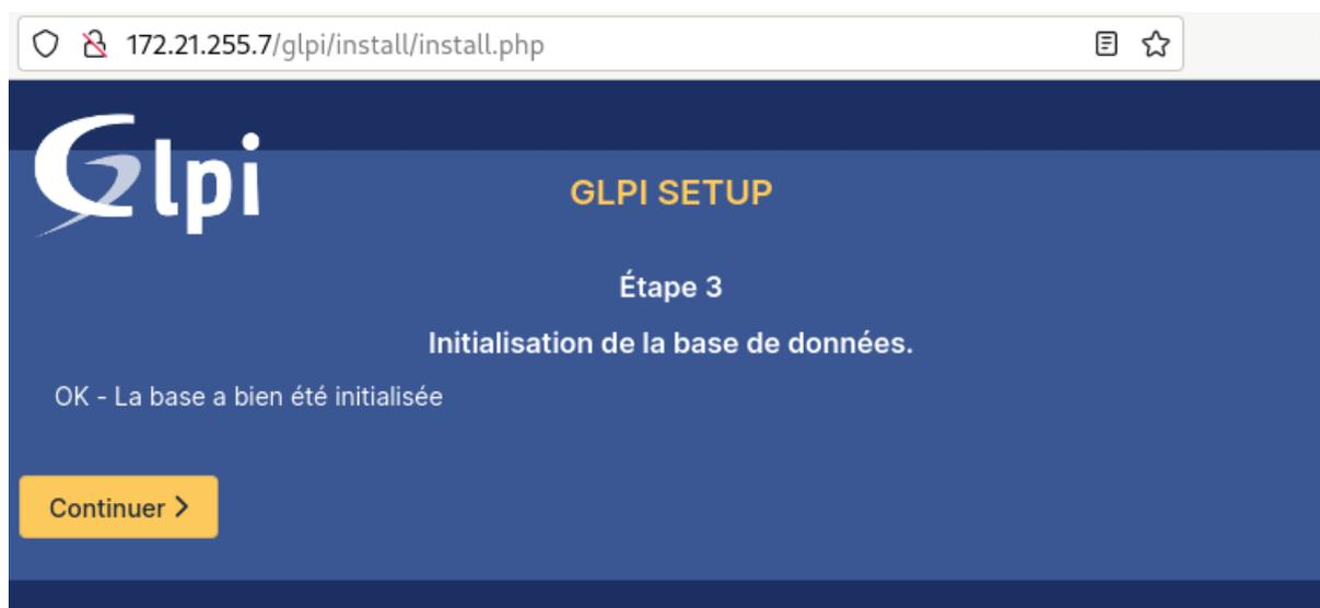
The screenshot shows the next step in the GLPI installation setup. The heading is "GLPI SETUP" in yellow. The page is titled "Étape 3" (Step 3) and "Initialisation de la base de données." (Database initialization.). A message reads "OK - La base a bien été initialisée" (OK - The database has been successfully initialized). A yellow "Continuer >" (Continue) button is at the bottom.
